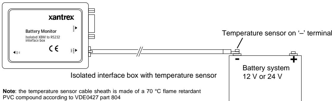
**Note:** the temperature sensor cable sheath is made of a 70 °C flame retardant PVC compound according to VDE0427 part 804
