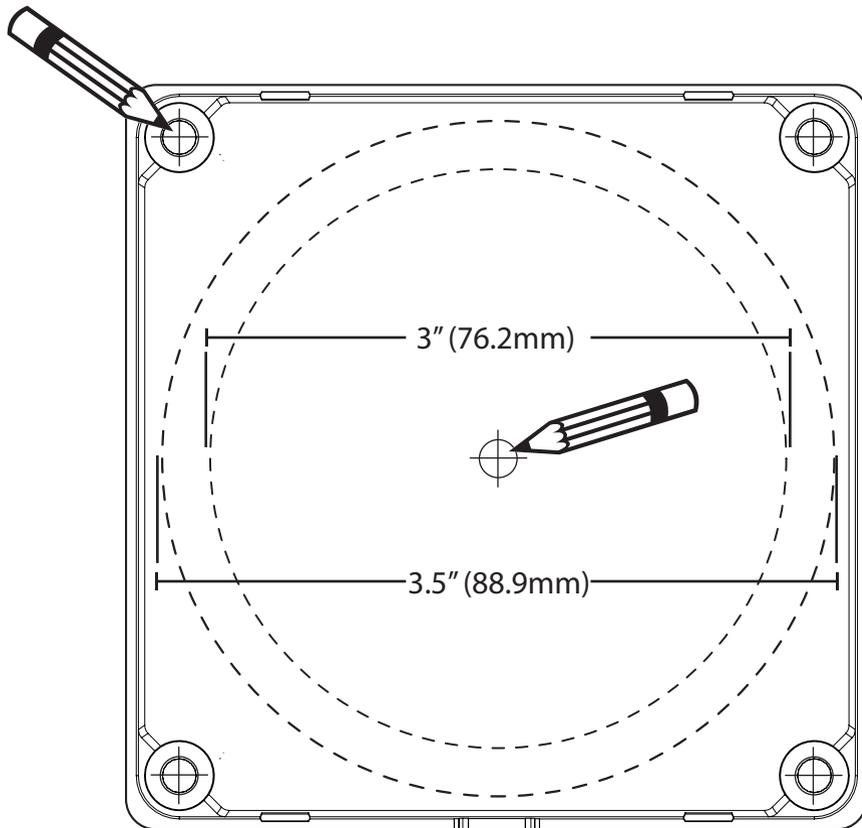
**NOTE:** Mark the positions of the center hole and the mounting holes on the wall where you plan to mount the remote panel. Use a hole saw with a minimum diameter of 3" (76.2mm) and a maximum of 3.5" (88.9mm) to cut a circular hole on the wall.
