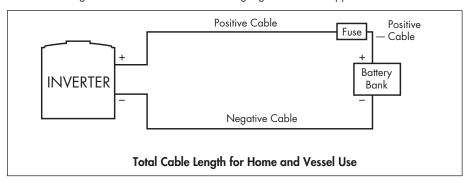
Many inverter installations are in 12V negative-ground vehicles. It is possible to use the vehicle frame as the part of the negative (-) conductor back to the battery or battery bank. To determine the Total Cable Length in this case, add all cable lengths. Do not include the vehicle chassis. If installing in vehicle, ground inverter to chassis. Do not ground inverter to negative terminal.
