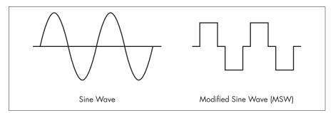
This modified sine wave has a root mean square (RMS) voltage of 115 volts. Most ordinary AC voltmeters are calibrated to read "average" voltage and assume that the AC waveform will be a pure sine wave. These meters will not correctly read MSW voltage, and will display about 20 to 30 volts too low. Any multi-meter identified as "TRUE RMS" will accurately read MSW correctly.
