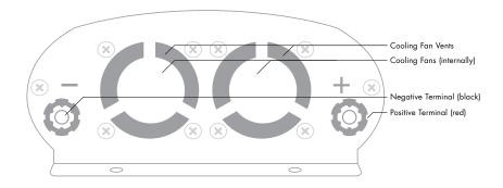
High Speed Fan – Keeps the inverter circuitry cool. The fan operates when the inverter is powered on. To avoid unnecessarily draining of the battery, turn off the inverter when it is not in use.
