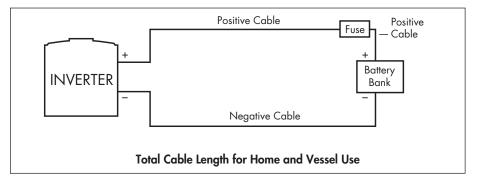
Many inverter installations are in 12V negative-ground vehicles. It is possible to use the vehicle frame as the part of the negative (-) conductor back to the battery or battery bank. To determine the Total Cable Length in this case, add all cable lengths. Do not include the vehicle chassis.
