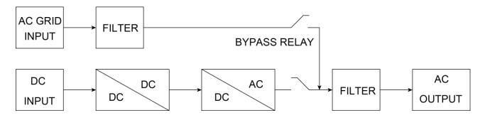
The inverter features IGBT technology which, minimizes weight and dimensions while enhancing output short circuit reliability and overload capacity. AC output voltage is provided in one of the two modes :
