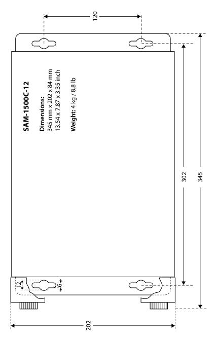
Fig 3.2 Dimensions & Mounting Arrangement
