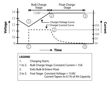
Fig. 2.2 Battery Charger Stages and Voltage/Current Curves
