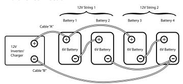
Fig. 4.4 Series-Parallel Connection
