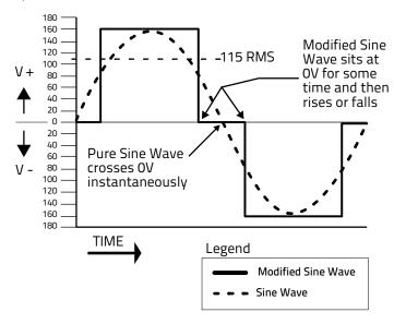
Fig 2.1 Modified Sine Wave and Pure Sine Wave - Comparison
