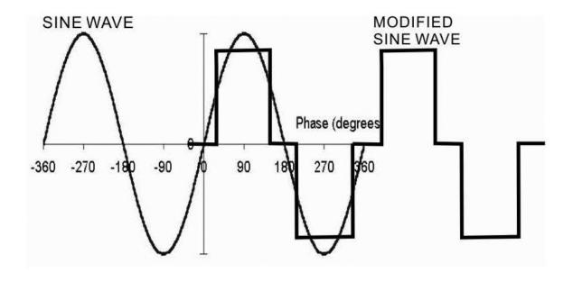
FIGURE 1: Modified Sine Wave and Sine Wave Comparison
