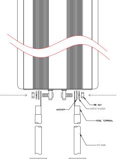
Do not place anything between battery cable lug and terminal surface. Assemble exactly as shown.
