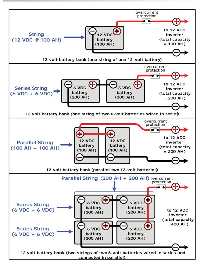
Figure B-4, Battery Bank Wiring Examples (12-volt)
