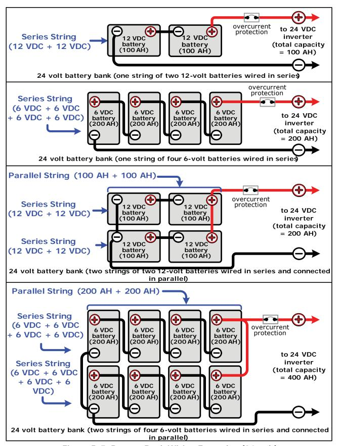
Figure B-5, Battery Bank Wiring Examples (24-volt)
