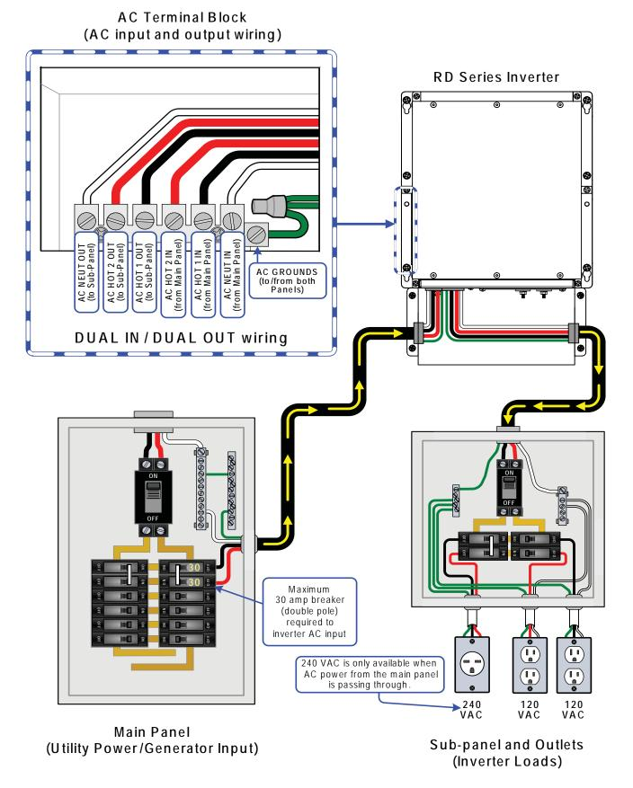
Figure 2-14, AC Wiring for Dual In - Dual Out Configurations
