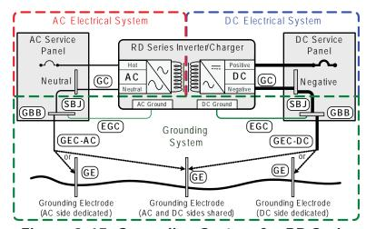
Figure 2-15, Grounding System for RD Series
