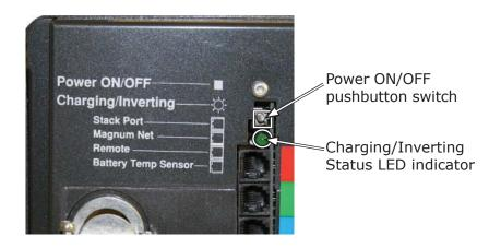
Figure 3-5, Power Switch and Status Indicator
