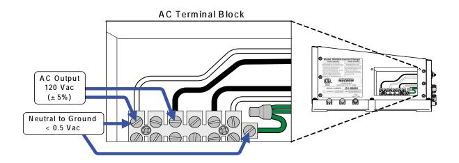
Figure 2-20, AC Voltage Checks
