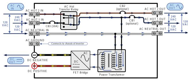
Figure 3-2, Power Flow - Standby Mode
