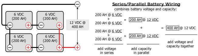
Figure B-3, Series-Parallel Battery Wiring
