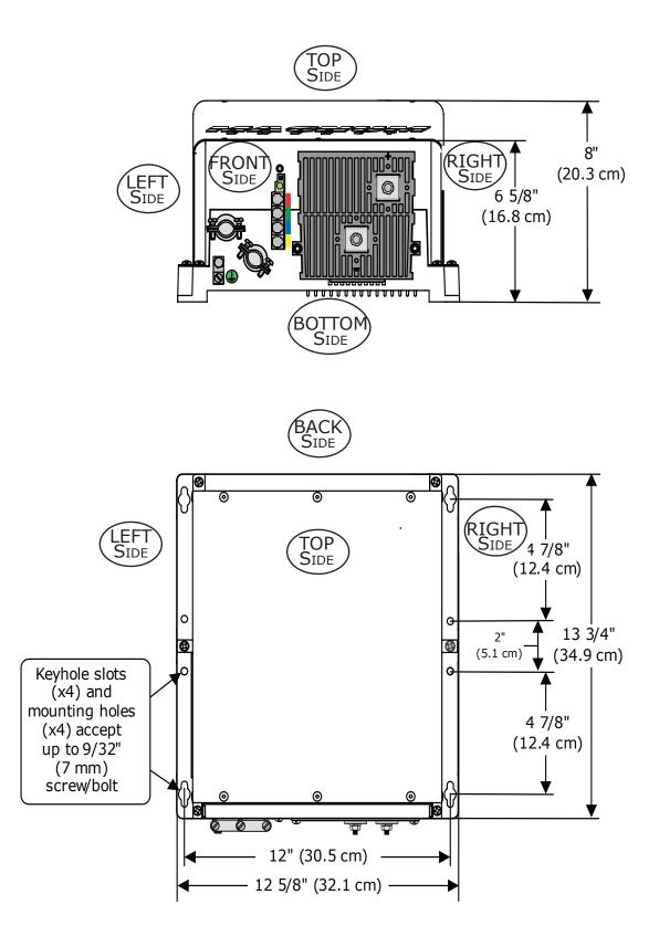
Figure 2-3, RD Series Dimensions and Side Reference
