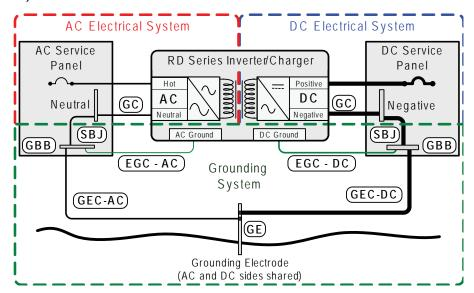
Figure 2-17, Multiple Connections to DC Ground Rod (Method 2)
