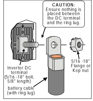
Figure 2-6, Inverter DC Hardware Installation
