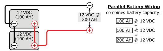
Figure B-2, Parallel Battery Wiring
