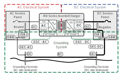
Figure 2-16, Multiple Connections to DC Ground Rod (Method 1)
