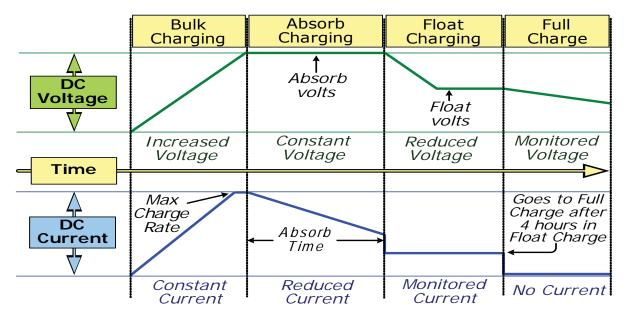
Figure 3-3, Automatic 4-Stage Charging Graph
