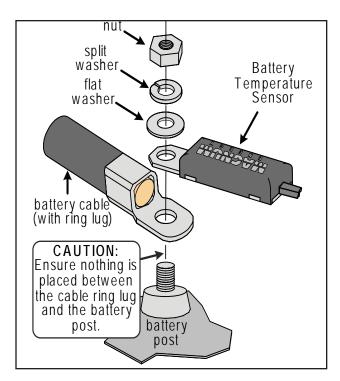
Figure 2-5, Battery Hardware Installation
