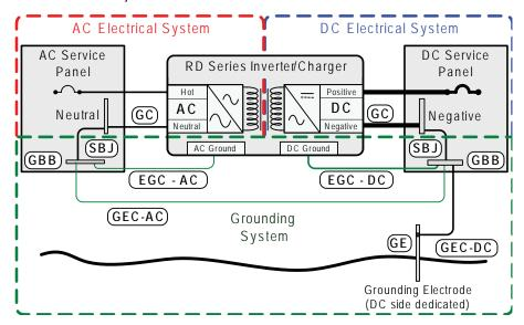
Figure 2-18, Single Connection to DC Ground Rod (Method 3)
