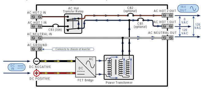
Figure 3-1, Power Flow - Inverter Mode
