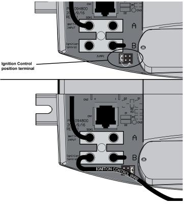
Figure 7 Exposed Ignition Control Terminals
