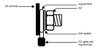
Figure 6 DC Cable Connections
