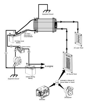
Figure 2 Typical Recreational Vehicle and Fleet Vehicle Installation
