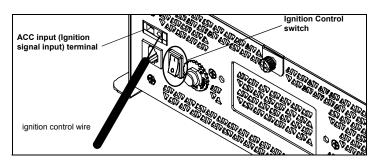
Figure 6 Ignition Signal (ACC) Input Terminal
