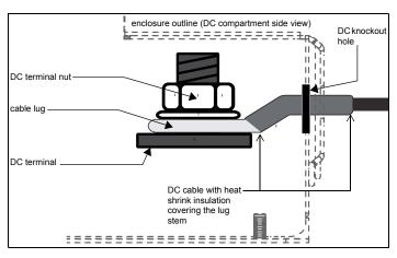
Figure 5 DC Cable Connections
