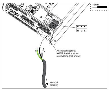
7. Locate the Neutral, Ground and Line terminals on the AC input terminal labeled as **N**, **G**, and **L** respectively.
