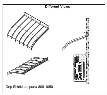
Figure 8 Drip Shields
