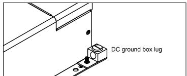
**Recreational Vehicle** Use 8AWG copper wire and connect it between the Chassis Ground lug and the vehicle's DC grounding point (usually the vehicle chassis or a dedicated DC ground bus).
