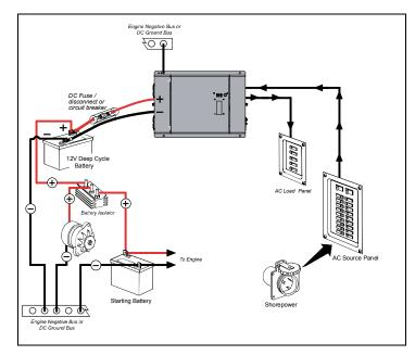
Figure 7 Typical Marine Installation
