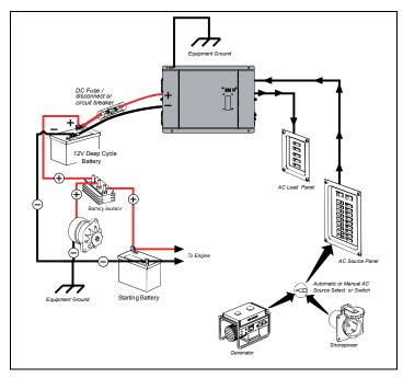
Figure 1 Typical Recreational Vehicle and Fleet Vehicle Installation
