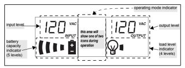
Figure 10 Parts of the LCD Screen
