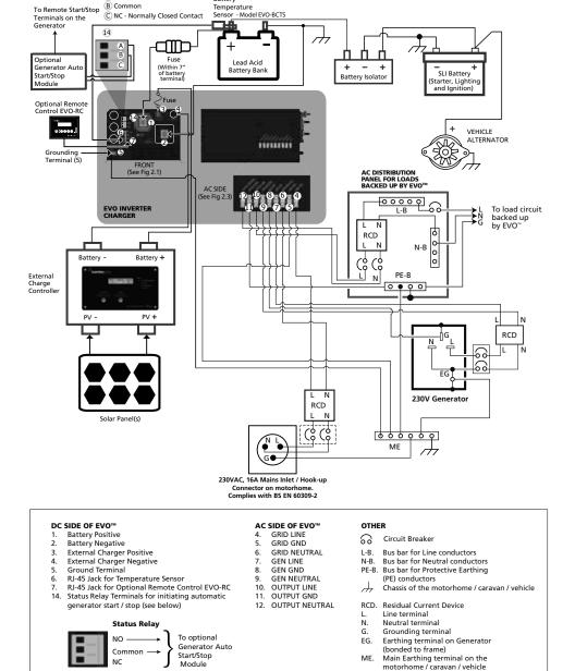
Fig 3.14 Typical Mobile Installation for Motorhome / Caravan / Vehicle
