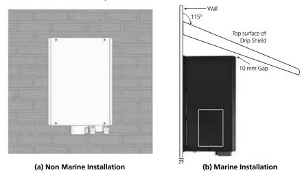
Fig 3.4 Mounting Arrangement 2: On Vertical Surface
