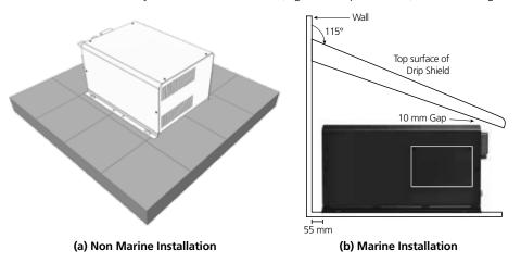
Fig 3.2 Mounting Arrangement: Horizontally On Horizontal Surface
