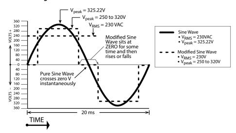
Fig 1.1 Pure and Modified Sine Waveforms for 230VAC, 50 Hz
