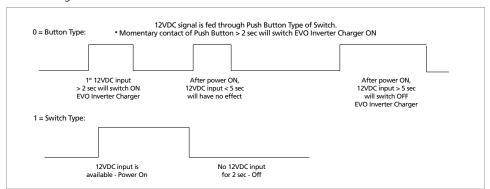
Fig 4.8. On/Off Logic Diagram for Remote Switch Options
