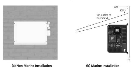
Fig 3.3 Mounting Arrangement 1: On Vertical Surface
