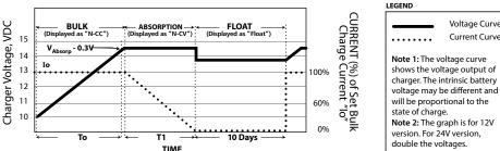
Fig 5.1 Charging Curve for Normal 3 Stage Charging
