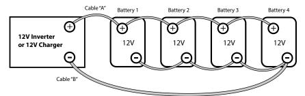
Fig 3.6 Parallel Connection
