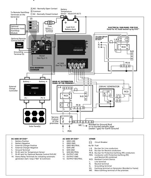
Fig 3.13 Typical Shore Based Installation for TN-C-S / Protective Multiple Earthing (PME) Distribution System
