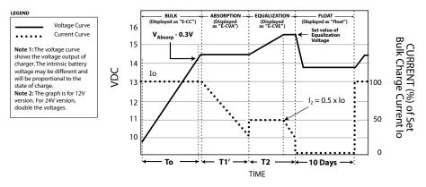
Fig 5.2 Charging Curve for 4 Stage Charging in Equalization Mode
