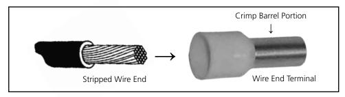
Fig 3.11 Stripped Wire End Terminal on AC Wiring
