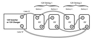
Fig. 3.7 Series-Parallel Connection
