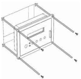
Flush mounting the EVO-RC on the wall with 4pcs, Φ3mm self-tapping screws (flat head).
