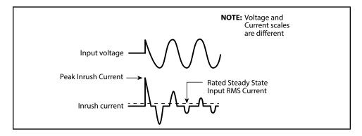
Fig 1.2 Inrush current in an SMPS
