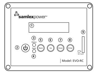
Fig. 1.1(a) Optional Remote Control EVO-RC - Layout
