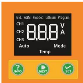
**CH1** - Display is showing the House Battery Bank info (charging voltage, current, and status)
